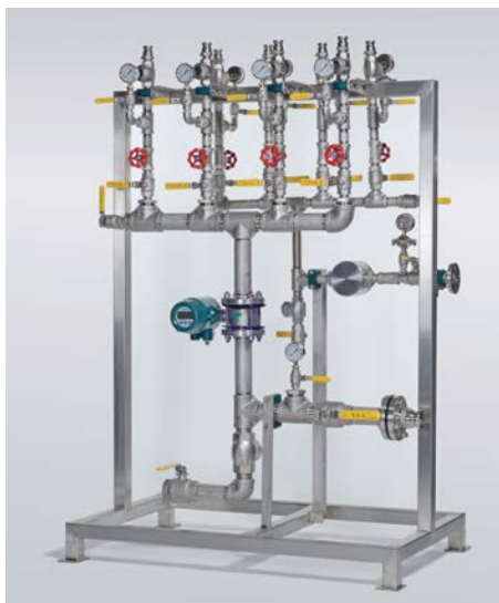
Dilution module controls white water and polymer flows.
